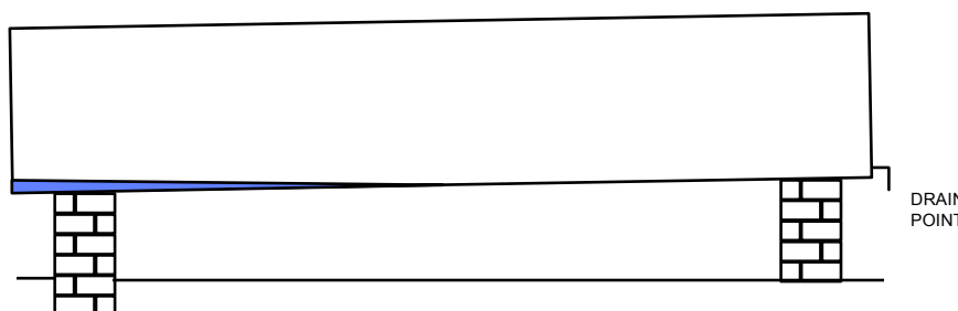
Figure 2 : Water and sediment cannot be drained
