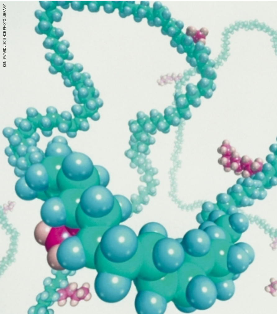
Linear low density polyethylene (LLDPE) consists of long chains of carbon and hydrogen atoms with short side chain branches. This structure gives the material good tensile strength, making it ideal for applications including films, sheeting and bags
