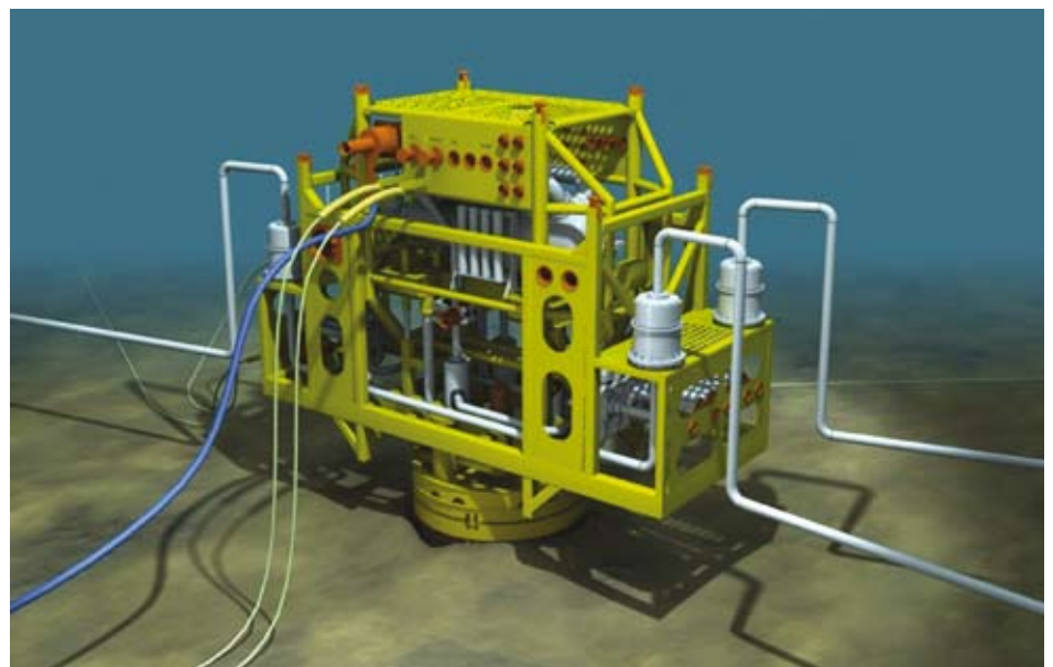
Each subsea pump station is 9 metres long by 8 metres high, weighs 88 tonnes and is mounted on a foundation pile in the seabed
