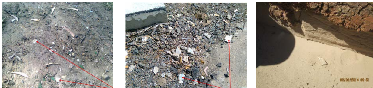
Examples of asbestos contamination of soil
