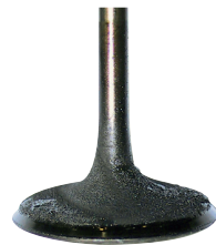
Fuel inlet valve using ordinary fuel* after 3200km
