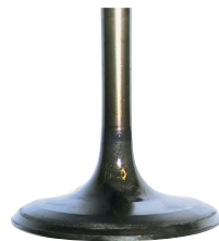
Fuel inlet valve using Opal fuel* after 3200km
