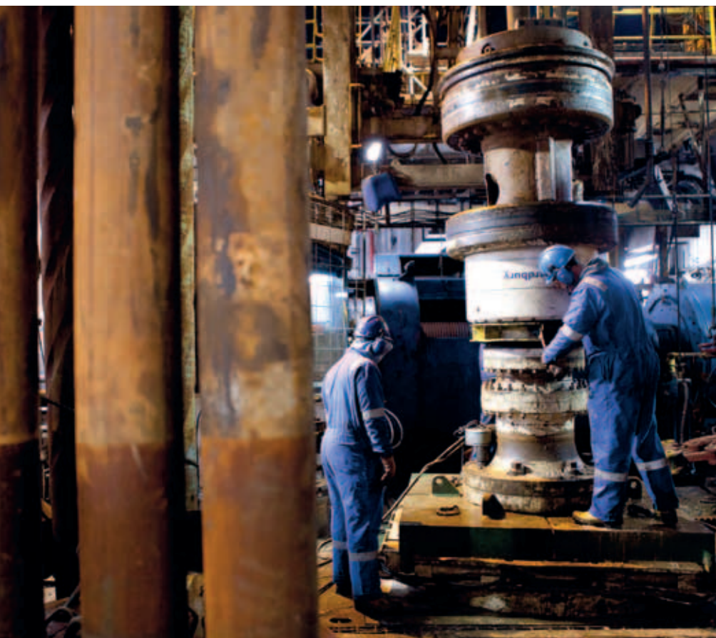
Offshore life: drilling engineer Claire Horsman (far left) carries out derrick inspection onboard the Byford Dolphin drilling rig. Offshore staff run the diverter – used to direct fluid – on the Byford Dolphin.
