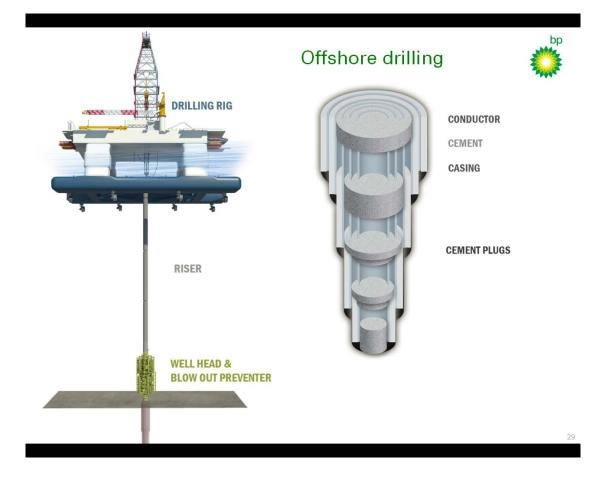
First we deploy a large diameter drill bit to the sea bed and drill the first section of the well.
