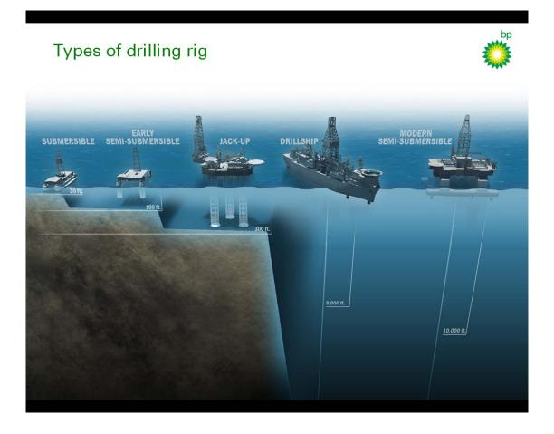
The first offshore rigs were submersibles with pontoons that were flooded with water and literally sat on the seabed.
