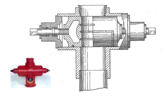
In 1924 along came an example of an innovation driven by risk management. This was the world's first successful blowout preventer, or BOP. It was a ram-type device, with simple hydrostatic pistons, fixed to the wellhead.
