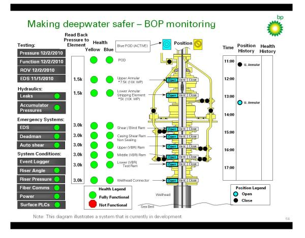
On deepwater rigs the status of each element of the BOP is monitored and we are now working on how that data might be presented using advanced diagnostic tools and an interface along the lines of the one shown here. This makes the data accessible in a new way to well site leaders and managers on shore as well as the engineers on the rig.
