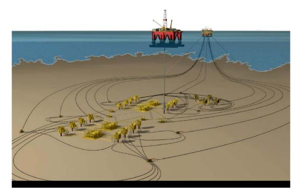
The production rig fabricated to produce oil from Atlantis is a 58,700-tonne semisubmersible platform which is tethered to the seabed over 7,000 feet below. For a few months in 2007 Atlantis was the deepest moored platform in the world.
