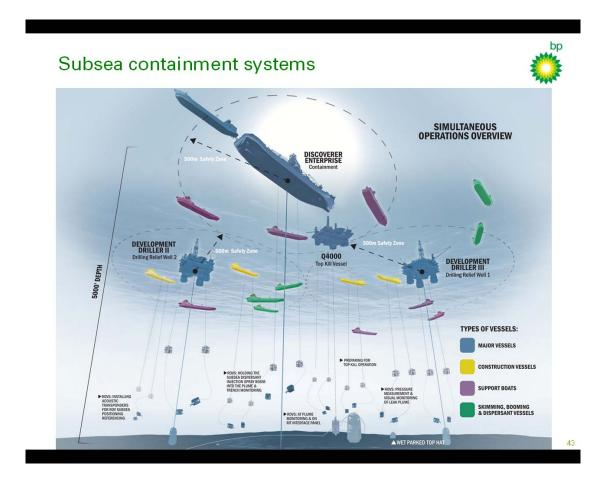
You can also see robot subs suspended from vessels at the surface. These were often moving around performing complex operations which had to be carefully choreographed in advance.
