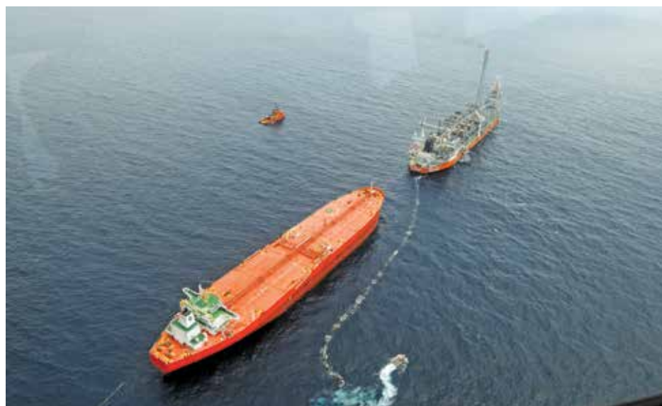
▲ Offloading operation in action at the FPSO PSVM terminal.
