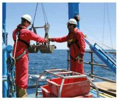
Collecting seabed sediment samples during offshore environmental survey
