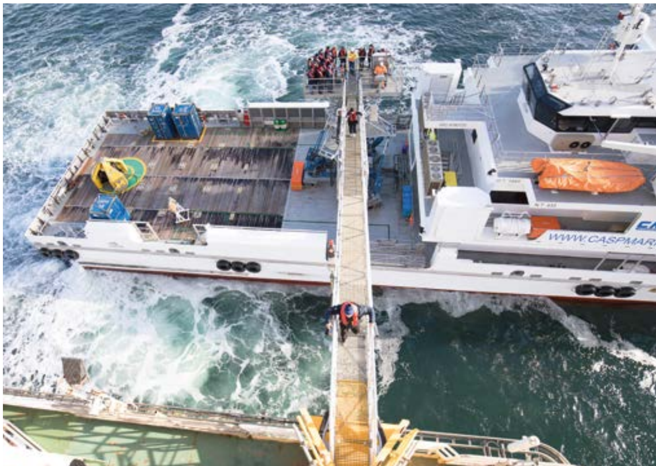
Our offshore employees use Ampelmann gangway connecting the crew change vessel to the platform to get to work safely.
