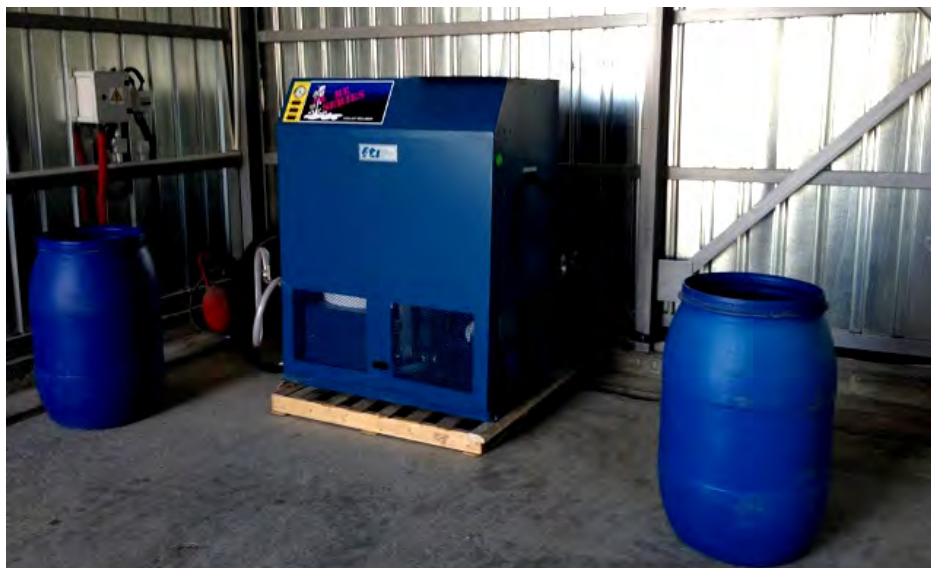
▲ Glycol recycler facility located at a pump station.
