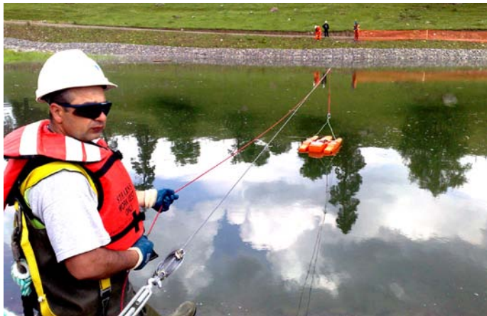
Secondary containment site velocity testing at Oshora river
