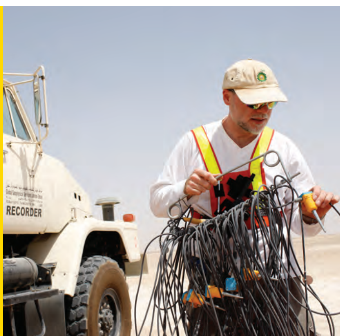
A geophysicist stands next to a vibrator truck, demonstrating the geophone system used to record vibration data over large areas of the desert within Block 61, Oman.
