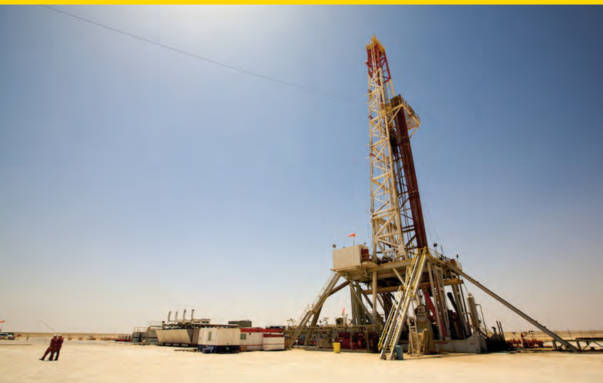
The Dalma LR5 rig, contracted to BP in Block 61, drilling one of BP's appraisal wells.
