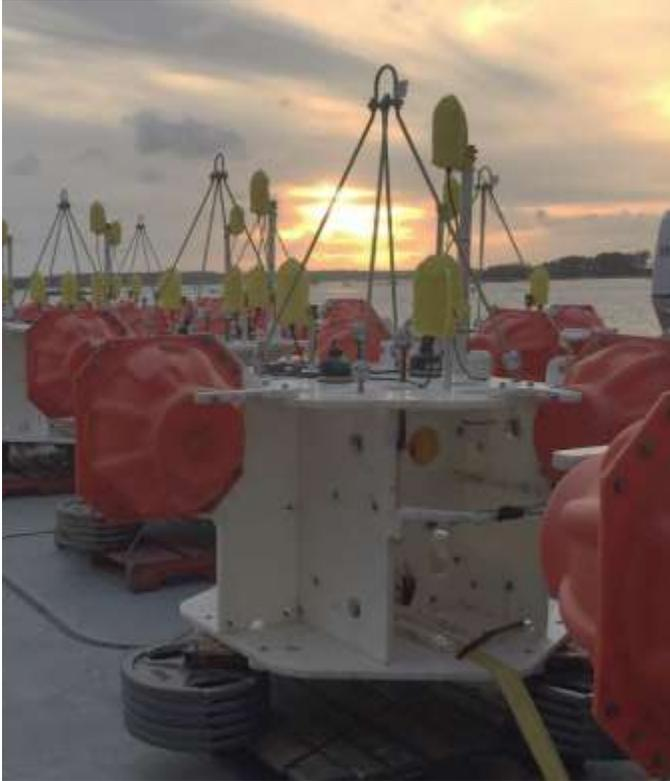
Figure A-2. Photo of ALTO landers prior to deployment. Each lander has an orthogonal array of four omnidirectional hydrophones spaced 50 cm apart (the hydrophones are inside the yellow flow shields). By using beamforming analysis methods, the direction of arrival of sounds can be determined from the four hydrophones. This configuration was used at ALTO1 and ALTO2 stations.
