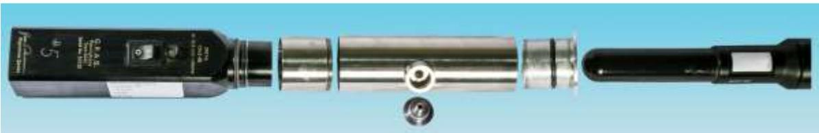
Figure A-3. Split view of a G.R.A.S. 42AC pistonphone calibrator with an M36 hydrophone.
