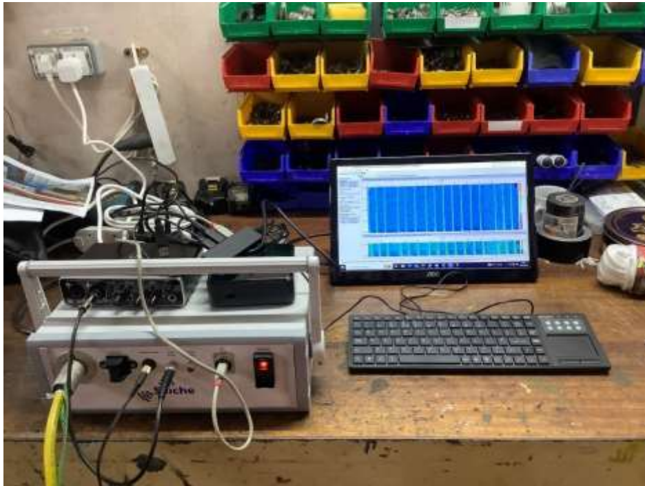
Figure 6-2: PAMGuard VSP Configuration - Hydrophone Tap Test Detections Displayed Across the Full Frequency Range of the Main Spectrogram Display
