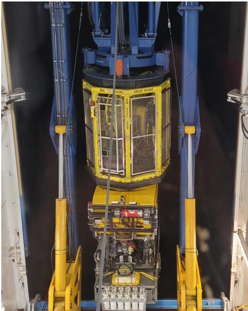
Figure 5-1: ROV with Push Core Rack Mounted on Sampling Skid
