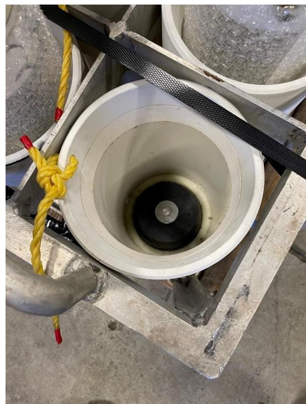
Figure 5-4: Push Core Holder with Base Plug
