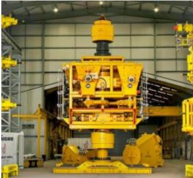
Figure 3: Well Control Capping Stack
