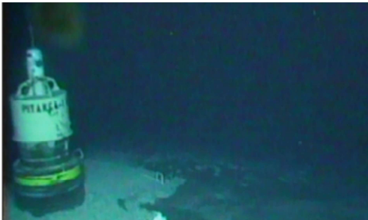
Underwater photo taken by ROV showing an abandoned wellhead on the seafloor
