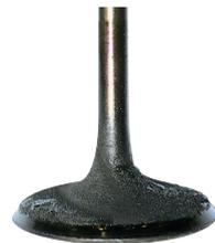
Fuel inlet valve using ordinary fuel\* after 3200km
