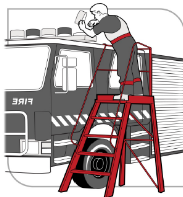
Figure 9 - A step platform can provide a stable work surface
