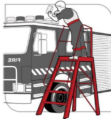
Figure 8 - A step platform can provide a stable work surface
