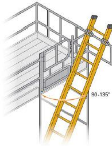
Figure 1 – angle of external scaffold ladders
