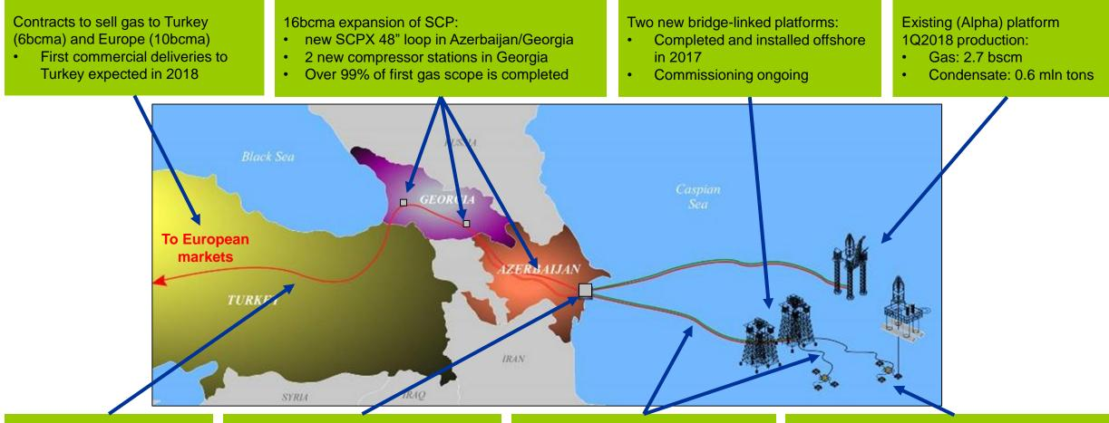
1,900km TANAP pipeline (not operated by BP) across Turkey New gas and condensate processing facilities with export gas compression at Sangachal now operational with hydrocarbons introduced into the system
