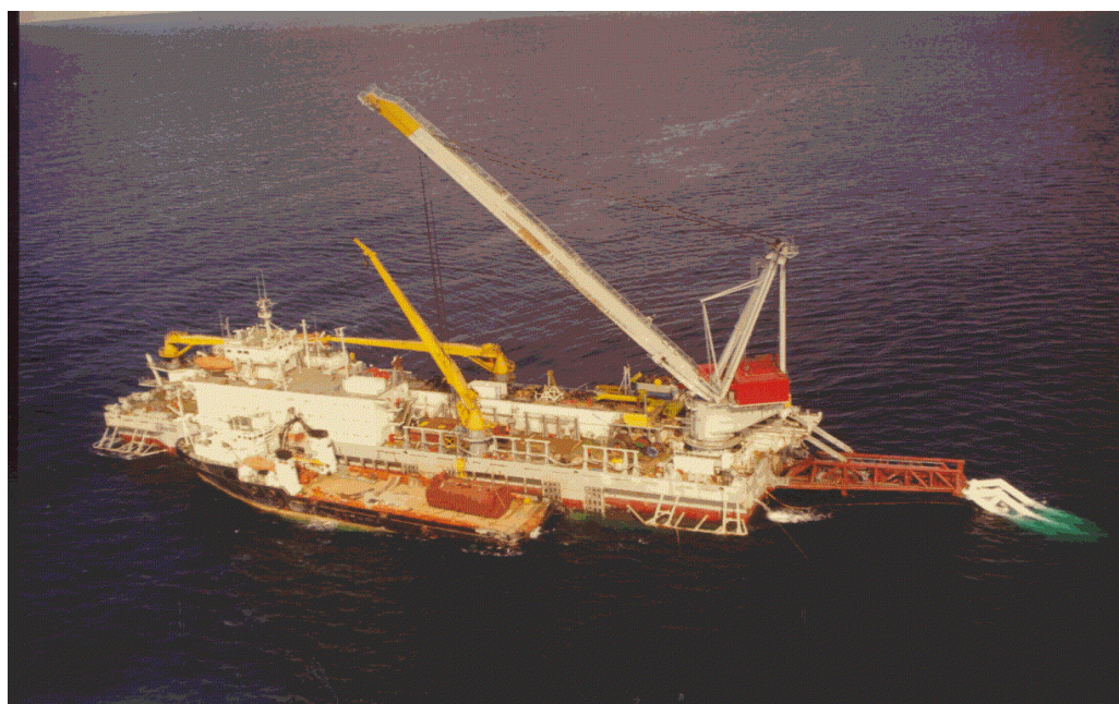
Figure 5.39 Pipelay barge, Israfil Guseinov
