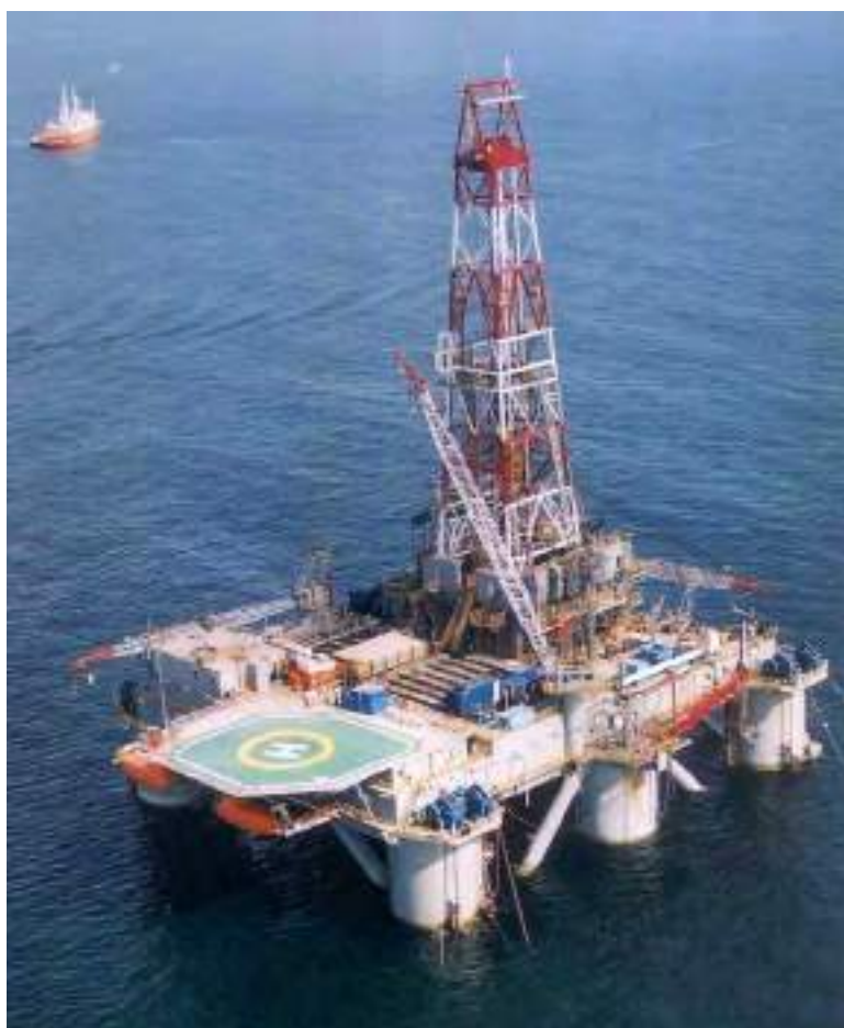
Figure 0.9: The Dada Gorgud Semi-submersible Drilling Rig
