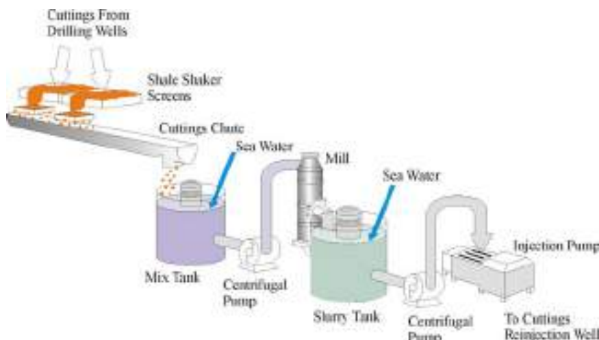
Figure 5.20 Cuttings Re-injection Process
