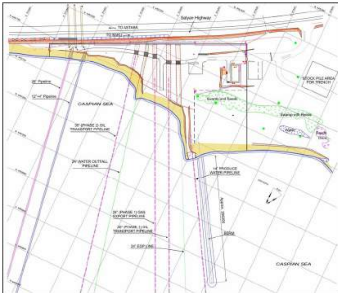
Figure 5.6 SD and ACG FFD PWD pipeline shore approach at landfall site
