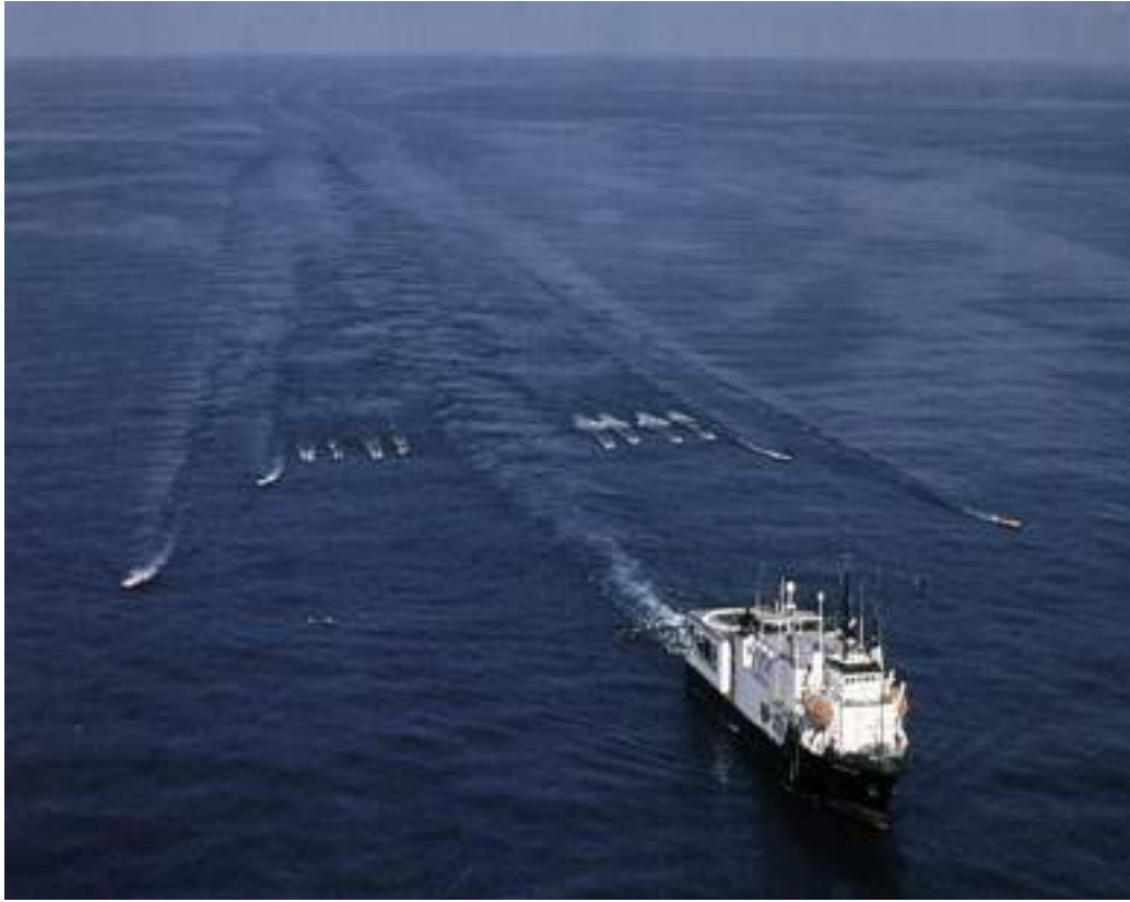
Figure 4.2: Example of Towed Streamer 3D Seismic Acquisition
