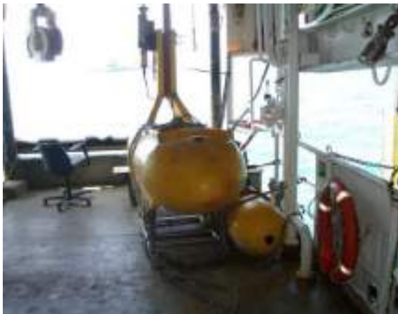
Figure 4.10: Deployment of a Tail Buoy Containing DGPS Receiver
