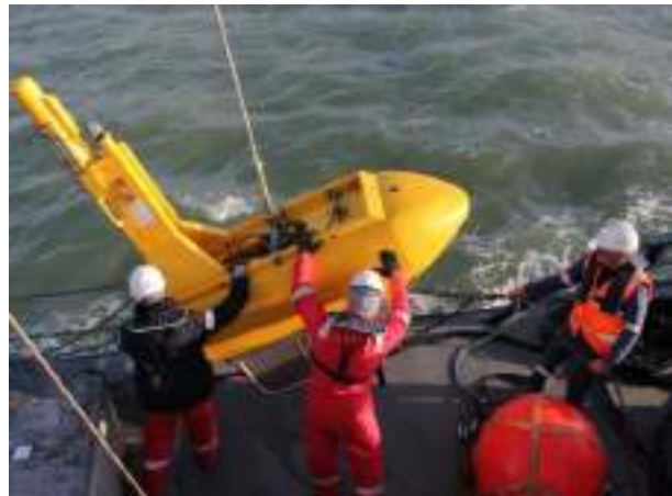
Figure 4.10: Deployment of a Tail Buoy Containing DGPS Receiver
