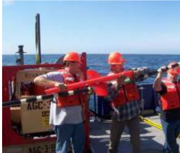
Figure 4.10: Deployment of a Tail Buoy Containing DGPS Receiver
