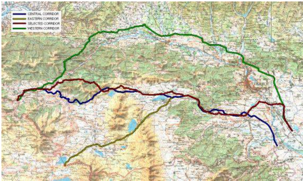
Figure 4-2 Alternative pipeline corridors through Georgia
