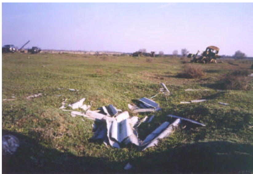
Figure 2 Surface contamination (suspected asbestos tiles)
