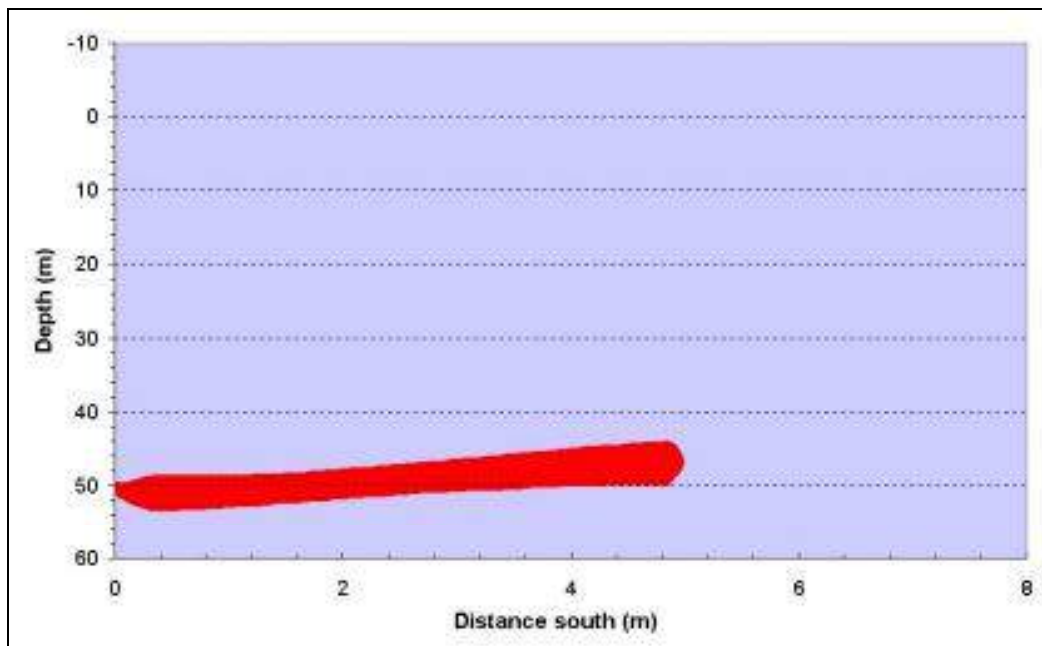
Figure 23: Shows the plume trajectory, to within 1°C of ambient temperature, as a function of depth and distance when released vertically from a 50m depth during summer.
