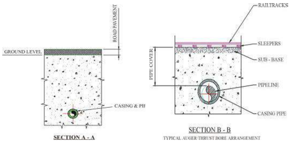
Figure 5.35 Pipeline service crossing method
