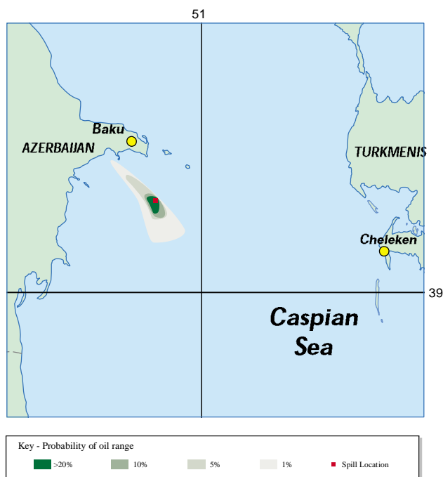
Figure 6b: Offshore Pipeline Leak 6899m 3 Azeri Condensate - Winter Conditions (357.72m 3 per hour for 19 hours).
