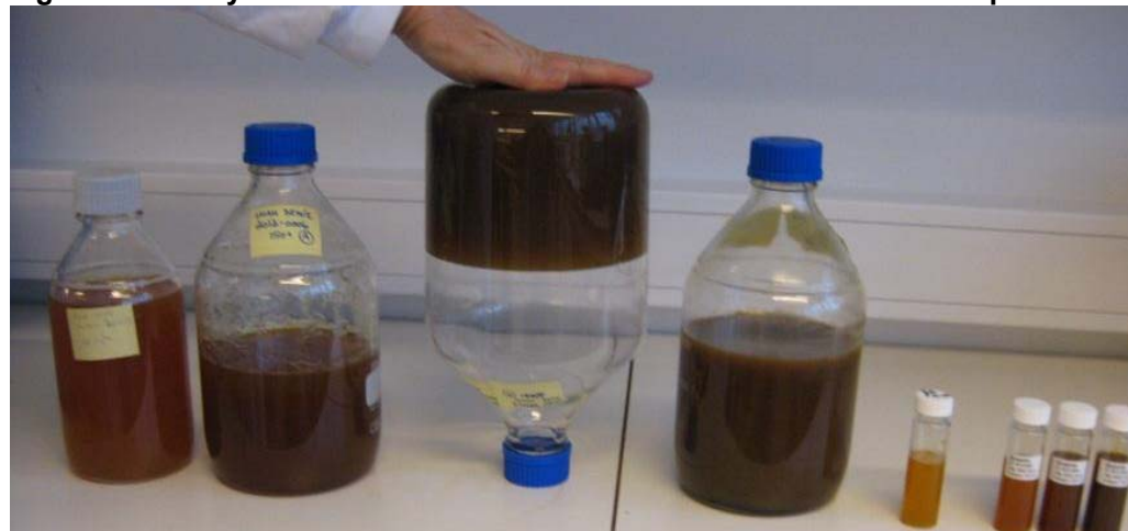
Figure 13.18 Physical State of the Distillation Residues at a Room Temperature Of 24°C
