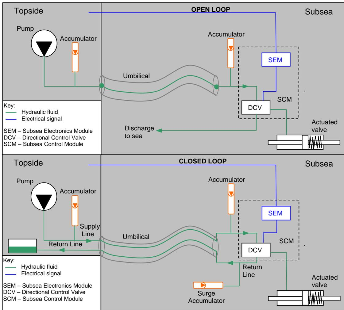
In an open loop system, discharge to sea occurs when the spring within the actuated valve returns the valve to the closed position, forcing the control fluid to discharge to sea. In a closed loop system hydraulic fluids are not discharged but are transferred back to the topside via return lines. In addition to the hydraulic fluid return line, the closed loop system also includes a surge accumulator; the function of which is to limit pressure build up in the return line.
