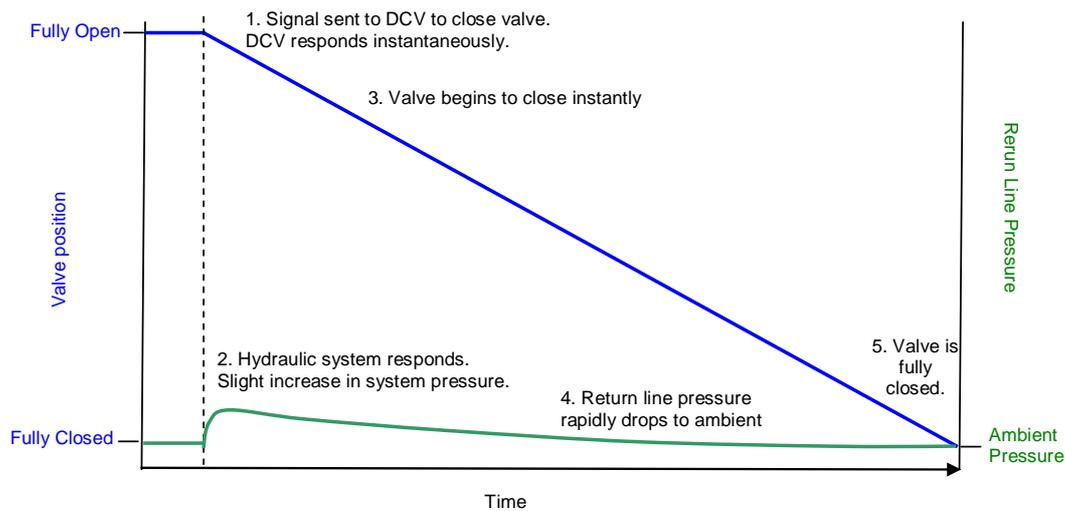
The figure shows that when the valve is operated there is an initial slight build up of back pressure within the system, which rapidly dissipates as the control fluid is discharged to sea. Modelling of the activities required to close the safety critical HIPPS valve showed that a closure time in the order of six seconds could be achieved for the open loop system.
