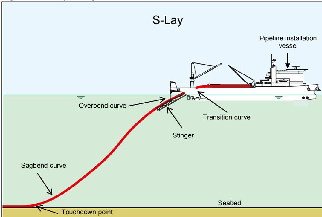
The 16” condensate line and 6” MEG line will be installed simultaneously. The 6” pipeline will be welded separately and the completed sections mechanically attached to the 16” pipeline using straps as it moves off the stern of the vessel.
