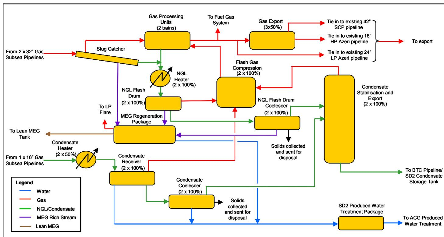
The SD2 onshore facilities are designed to incorporate two gas and condensate processing trains.
