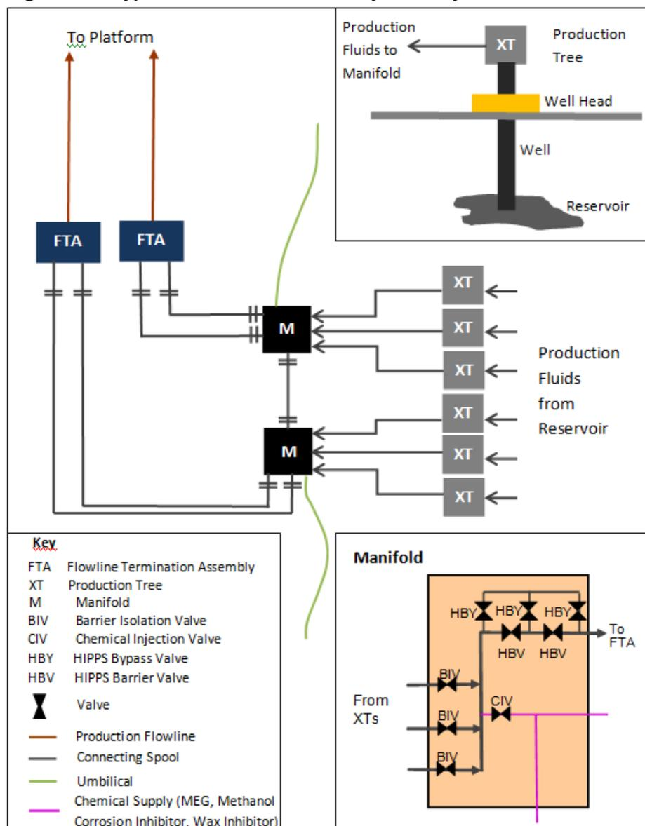
The subsea production system valves will be controlled from the SDB-QU platform using an open loop subsea control system. Chemicals and power required for flow assurance (i.e. wax, scale, corrosion and hydrate management) will be provided from the SDB-QU platform via umbilicals.
