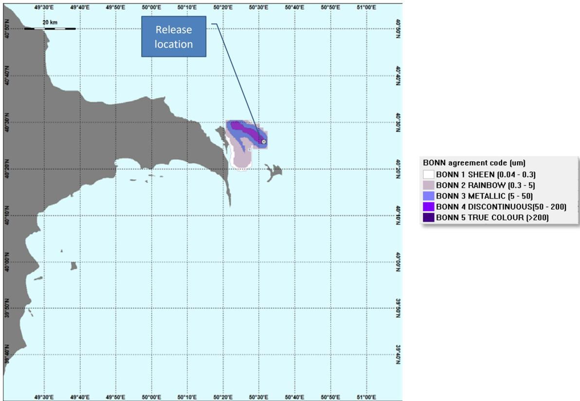
Figure 21: Diesel spill: Cumulative area of surface sheen - summer
