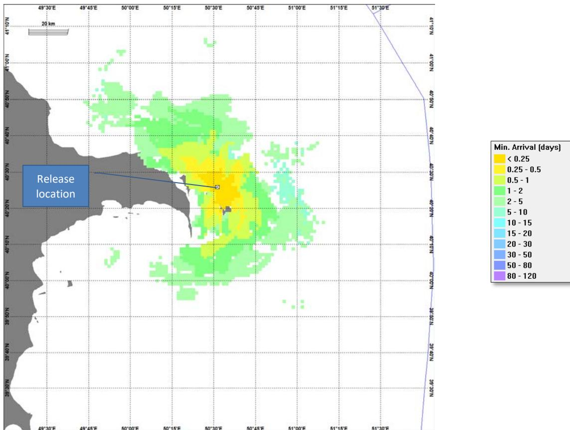
Figure 14: Diesel spill: Minimum arrival time of oil on surface (winter)
