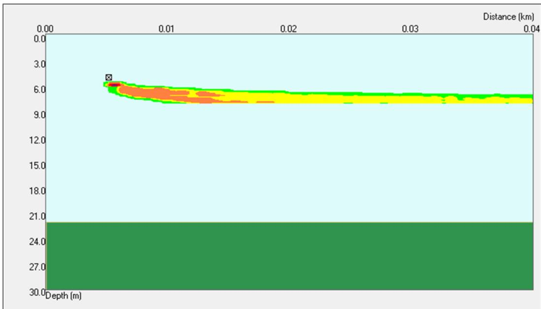
Figure 54: Stable thermal plume, summer, high current conditions (0.68 m/s)
