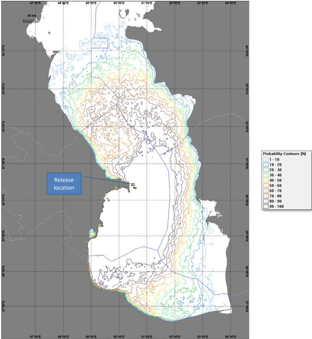
Figure 34: Worst case blowout: Probability of surface oil above threshold of 0.04 µm (winter)
