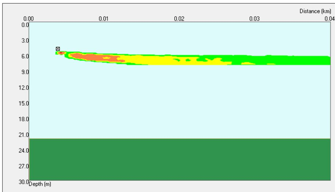
Figure 56: Stable thermal plume, winter, high current conditions (1.10 m/s)
