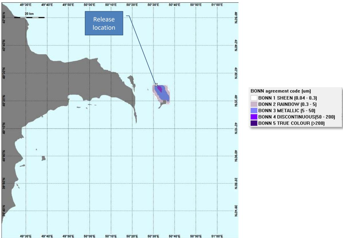
Figure 22: Diesel spill: Cumulative area of surface sheen - winter
