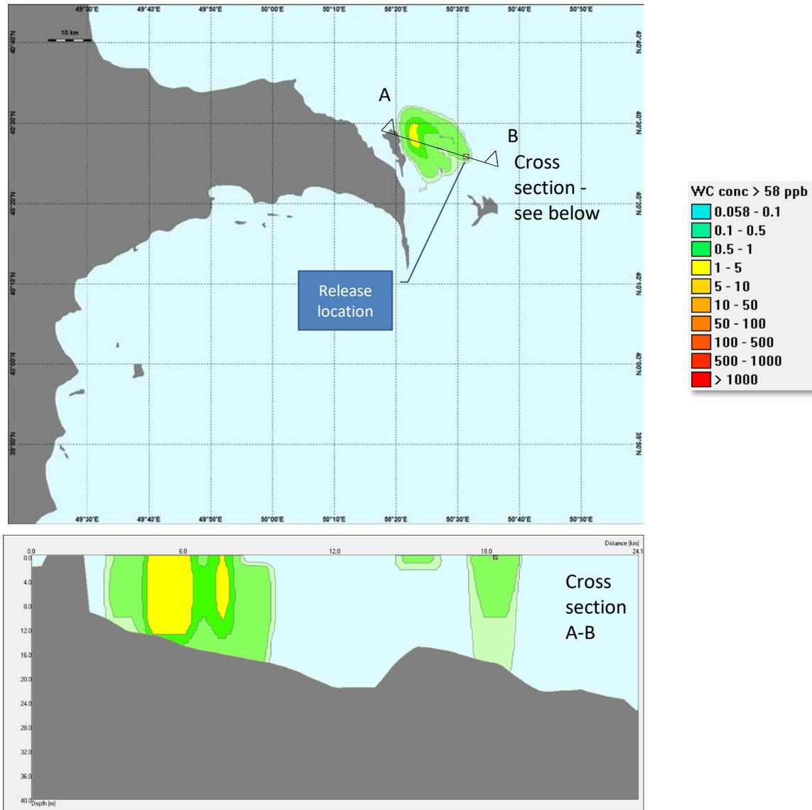
Figure 26: Diesel spill: maximum affected area of water column during simulation - summer
