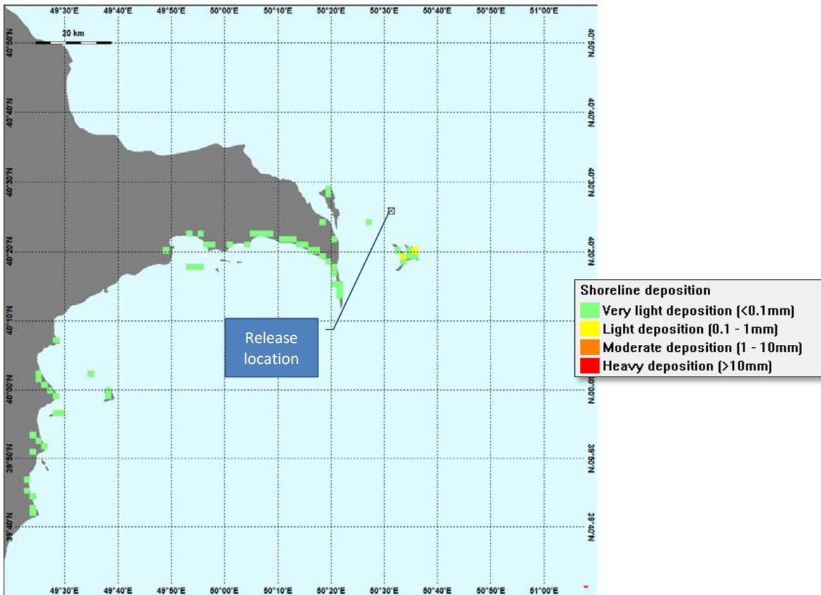
Figure 24: Diesel on shore - winter (length of shoreline affected at end of simulation)
