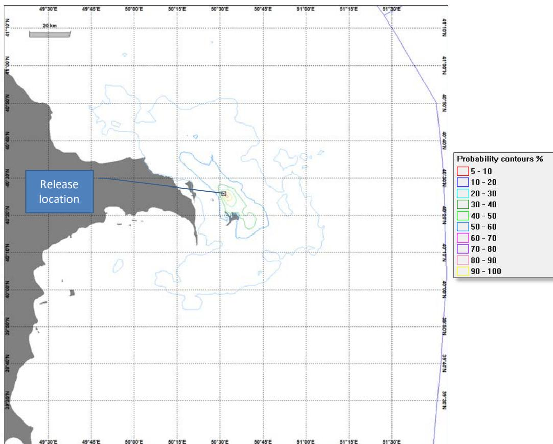
Figure 12: Diesel spill: Probability of surface oil above threshold of 0.04 µm (winter)
