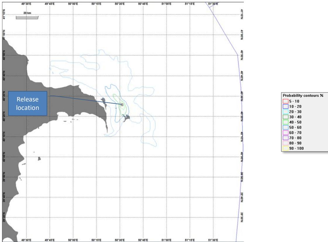
Figure 19: Diesel spill: Probability of oil in water column above threshold of 58 ppb (summer)
