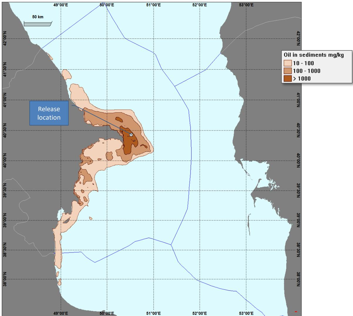
Figure 53: Worst case blowout: maximum mass of oil deposited in sediments (winter)
