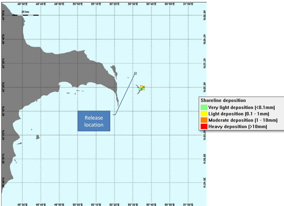
Figure 25: Diesel on shore - winter (maximum mass of diesel on shoreline)
