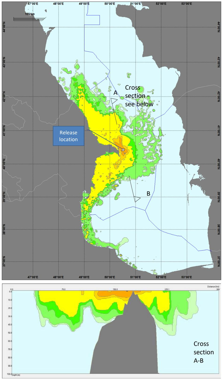
**Figure 50: Worst case blowout: maximum affected area of water column during simulation - summer**
