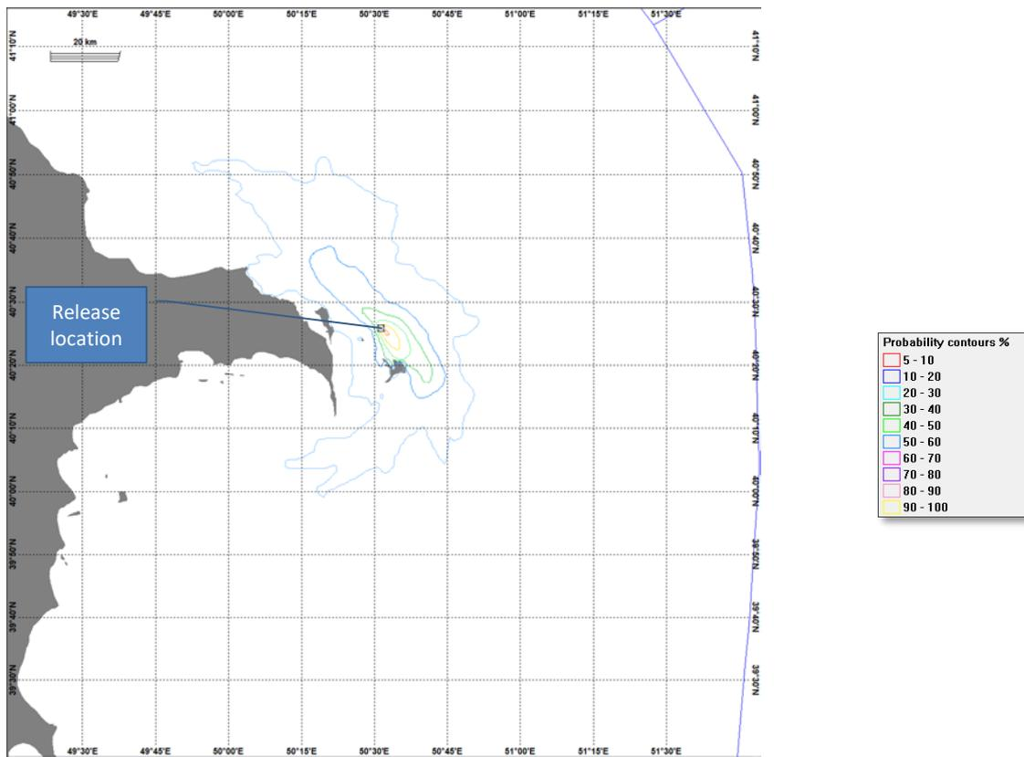
Figure 20: Diesel spill: Probability of oil in water column above threshold of 58 ppb (winter)
