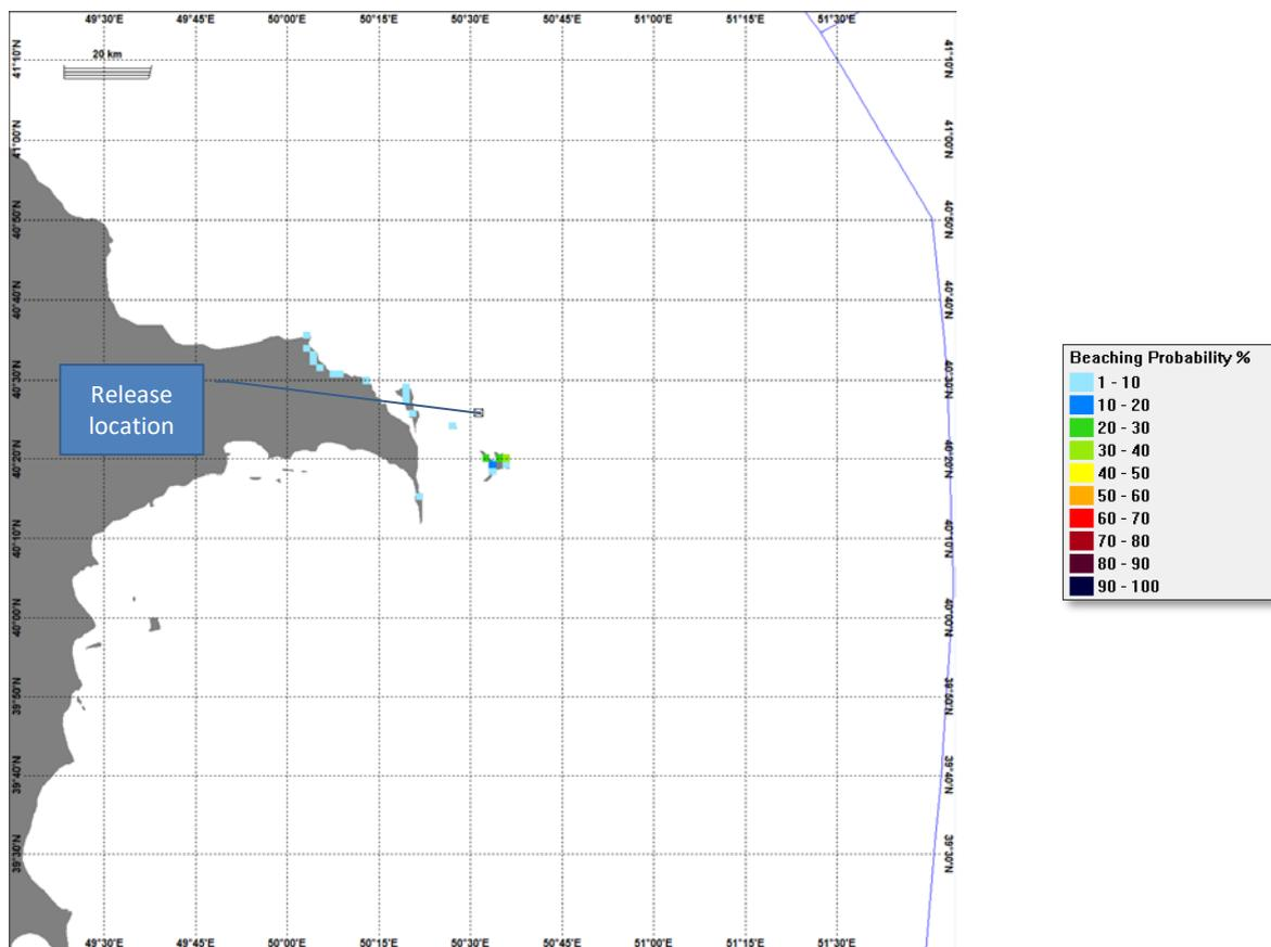
Figure 16: Diesel spill: Probability of oil on shoreline above threshold of 100 ml/m<sup>2</sup> (winter)
