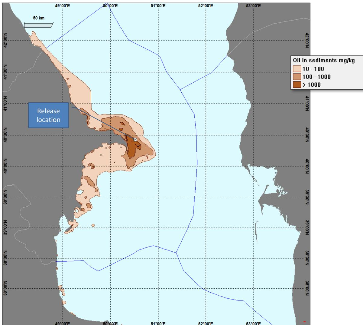
Figure 52: Worst case blowout: maximum mass of oil deposited in sediments (summer)
