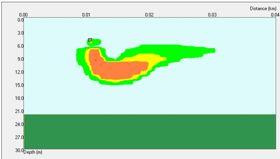
Figure 55: Stable thermal plume, summer, low current conditions (0.12 m/s)
