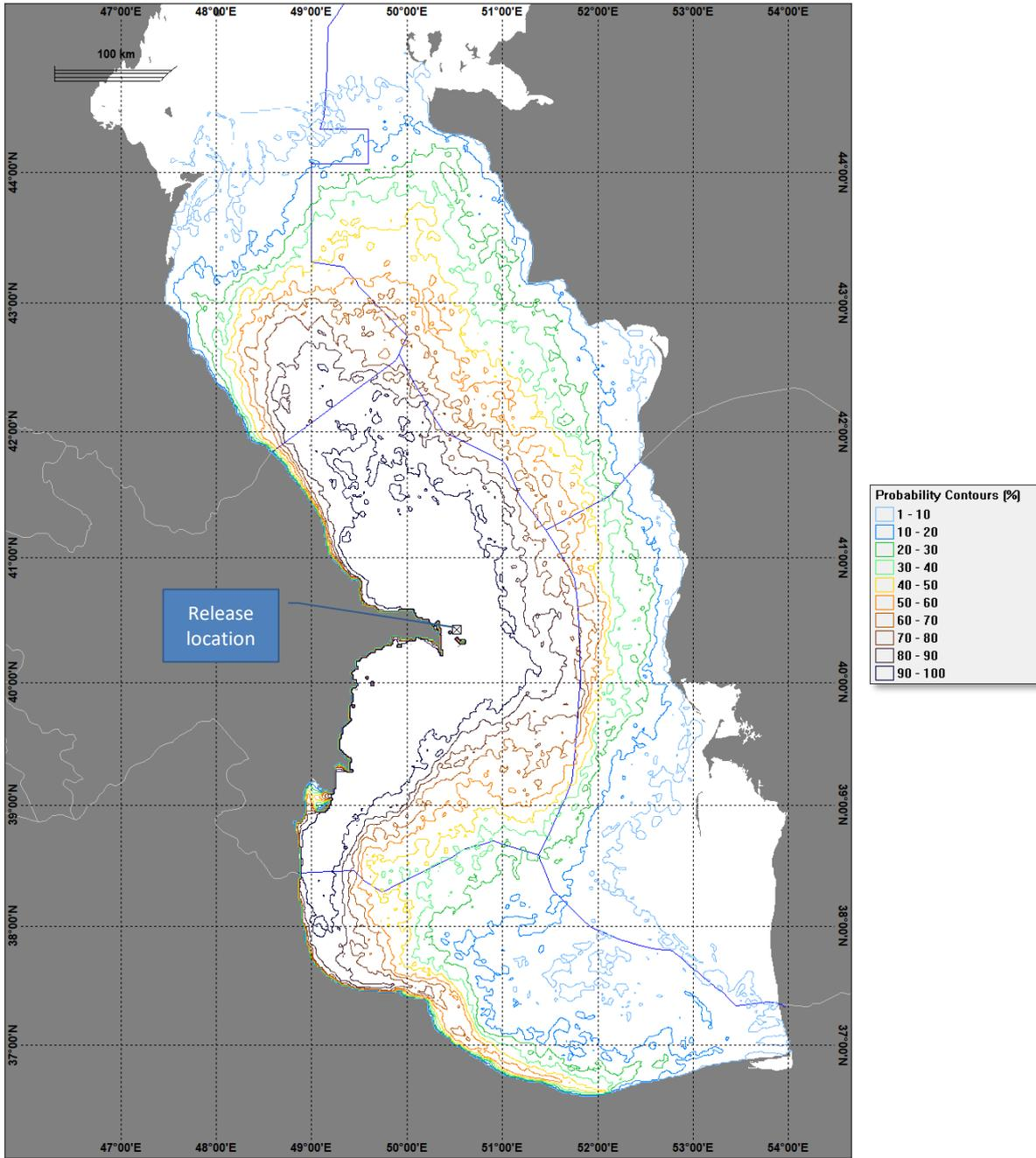
Figure 43: Worst case blowout: Probability of oil in water column above threshold of 58 ppb (summer)
