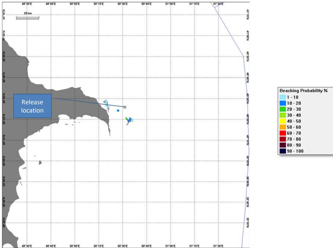
Figure 15: Diesel spill: Probability of oil on shoreline above threshold of 100 ml/m<sup>2</sup> (summer)
