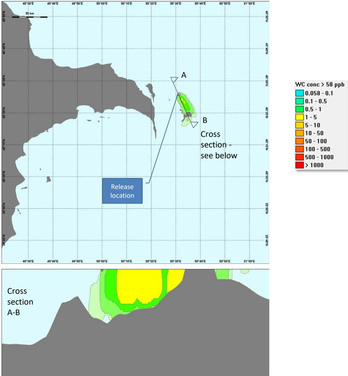
Figure 27: Diesel spill: maximum affected area of water column during simulation - winter
