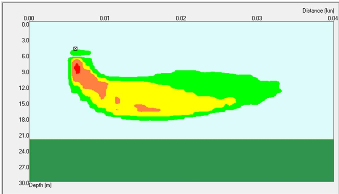
Figure 57: Stable thermal plume, winter, low current conditions (0.16 m/s)
