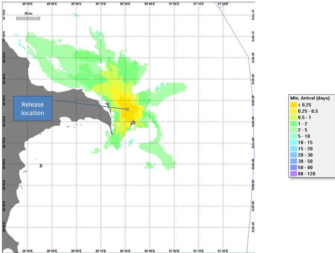
Figure 13: Diesel spill: Minimum arrival time of oil on surface (summer)
