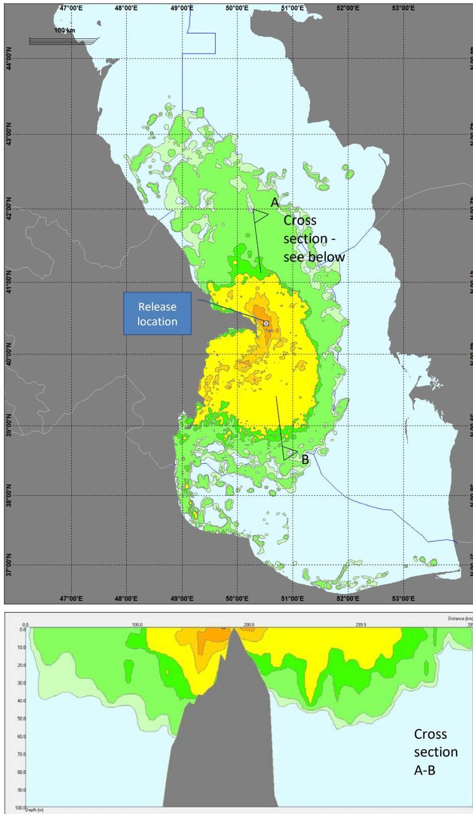
Figure 51: Worst case blowout: maximum affected area of water column during simulation - winter
