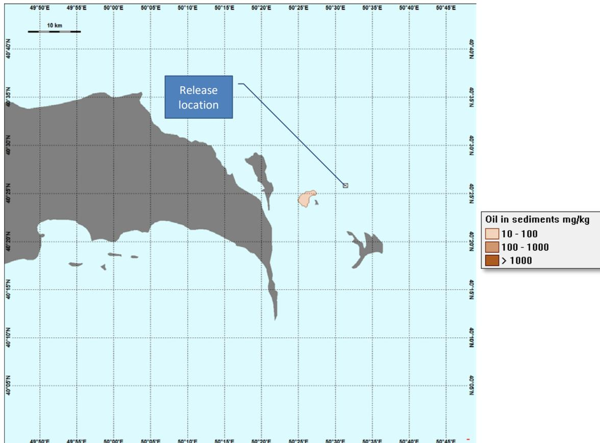
Figure 28: Worst case blowout: maximum mass of diesel deposited in sediments - summer
