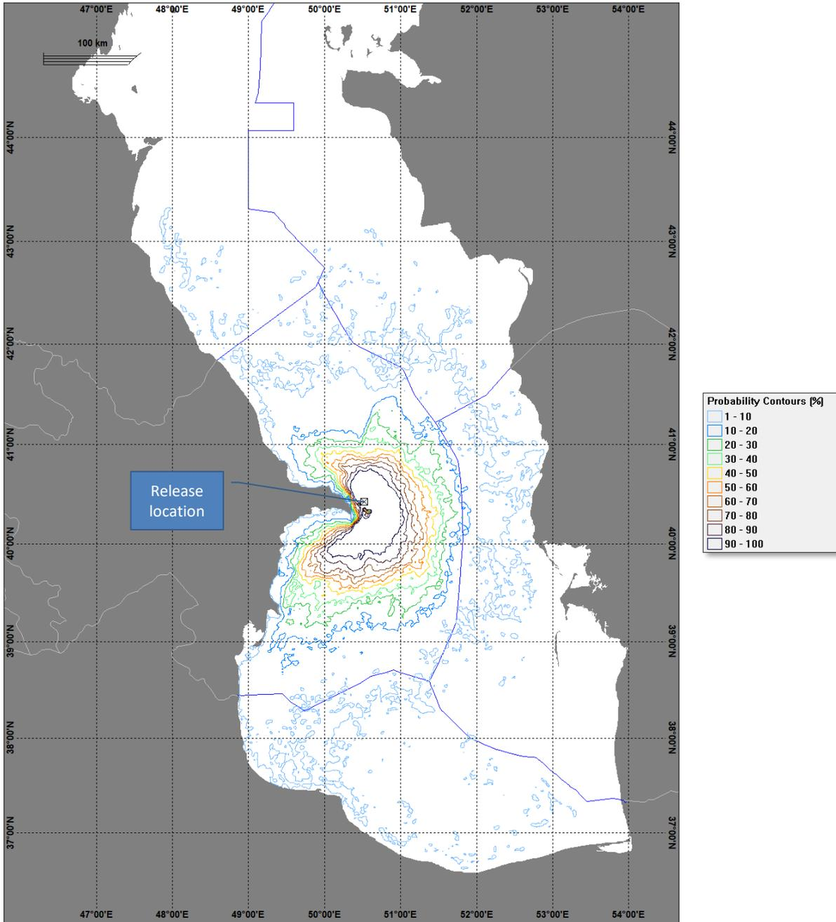
**Figure 44: Worst case blowout: Probability of oil in water column above threshold of 58 ppb (winter)**
