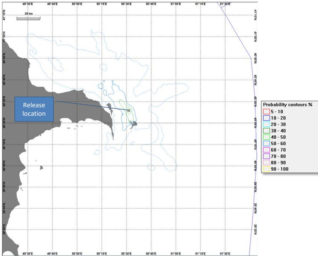
Figure 11: Diesel spill: Probability of surface oil above threshold of 0.04 µm (summer)
