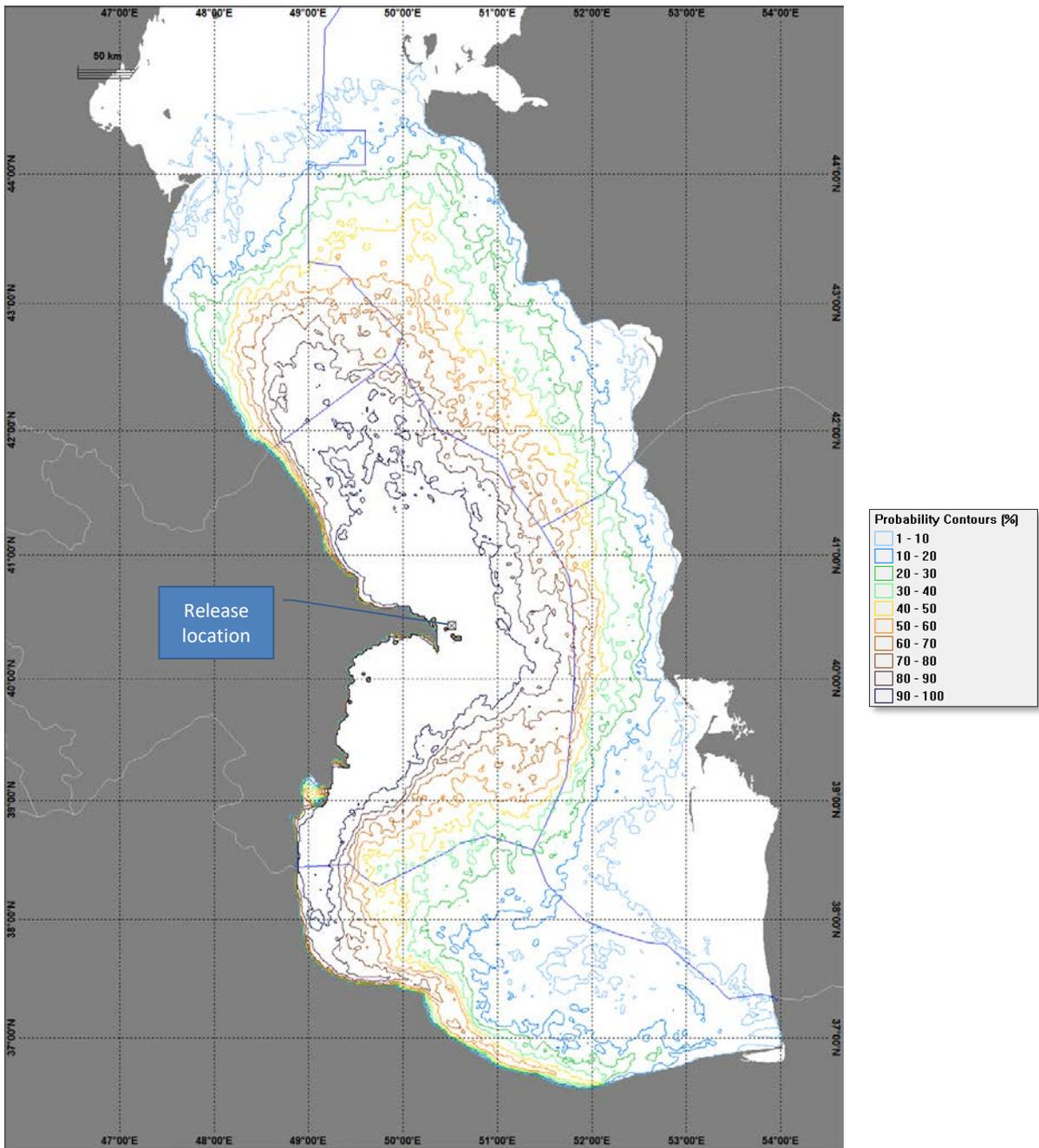
Figure 33: Worst case blowout: Probability of surface oil above threshold of 0.04 µm (summer)
