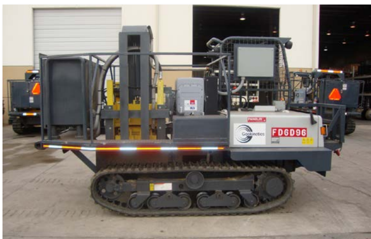
Figure E.3: Onshore Synchronised Electrical Impulsive Source Unit
