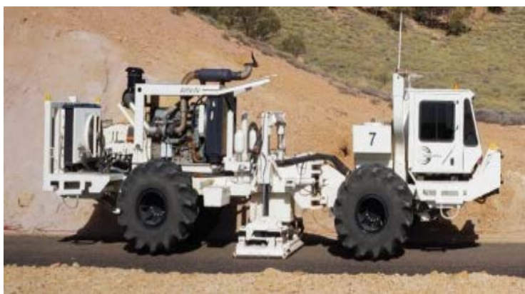
Figure E.3: Onshore Synchronised Electrical Impulsive Source Unit
