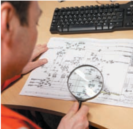
Confirming a valve number on a piping and instrument drawing for an isolation on DWG platform
