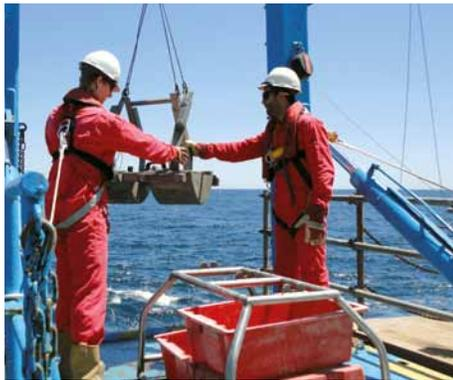
Collecting seabed sediment samples during offshore environmental survey
