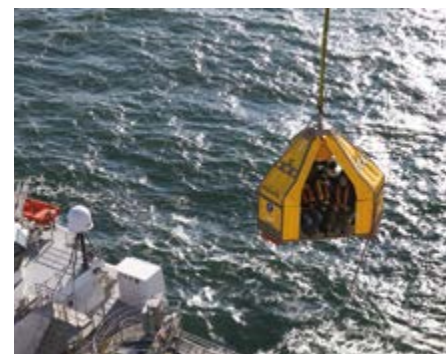
Frog is a crew transfer device with cutting-edge safety features, used to transfer employees from the vessel to the platform
