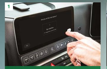
Once at the service station, the driver uses the In-Truck Connect app to locate and connect to the station via GPS
