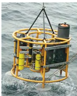
Figure 3-23 - Examples of seafloor lander designs deployed during the Strategies for Environmental Monitoring of Marine Carbon Capture and Storage (STEMM-CCS) project (NOC, 2022)
