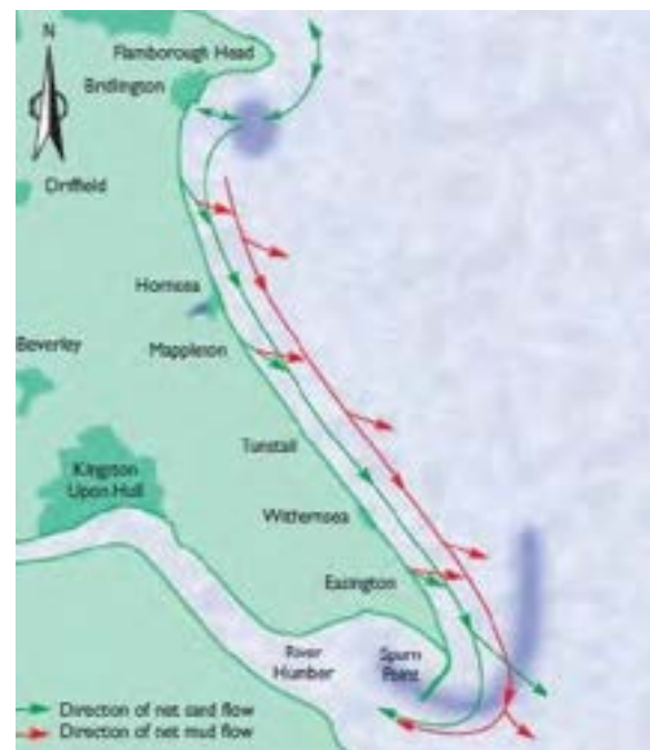
Figure 4-8 - Sediment transport figures demonstrating (a) dominant northeasterly wave direction which leads to net southerly movement of beach sand and (b) dominant offshore transport of eroded clay cliffs, bed strata bed strata and sand in suspension (ERYC, 2017a)
