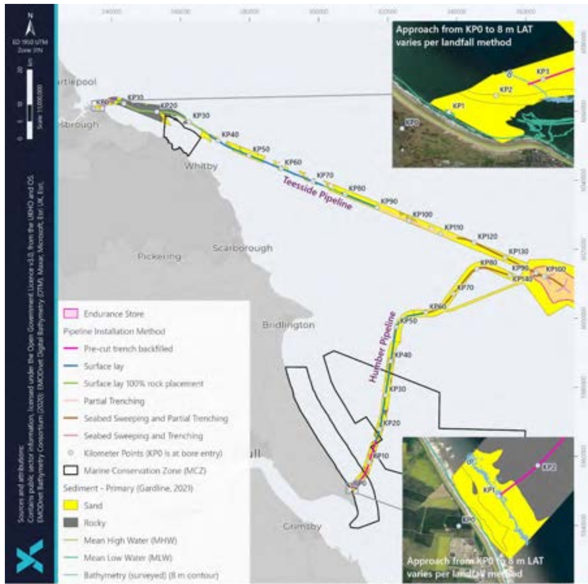
Figure 3-15 - Proposed installation methodology along the Teesside and the Humber Pipeline routes
