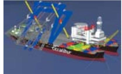
**Figure 7.2c:** Excalibur ‘single lift’ method (Ref. 7.15).
