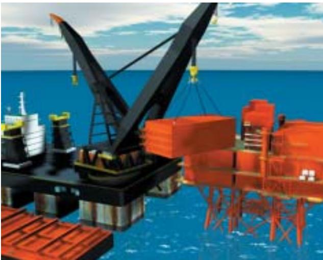
**3** Large module being lifted by heavy lift vessel
