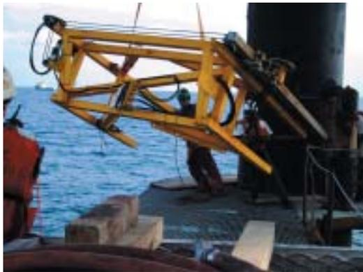
**Figure 8.5:** Photograph of a diamond wire cutter.
