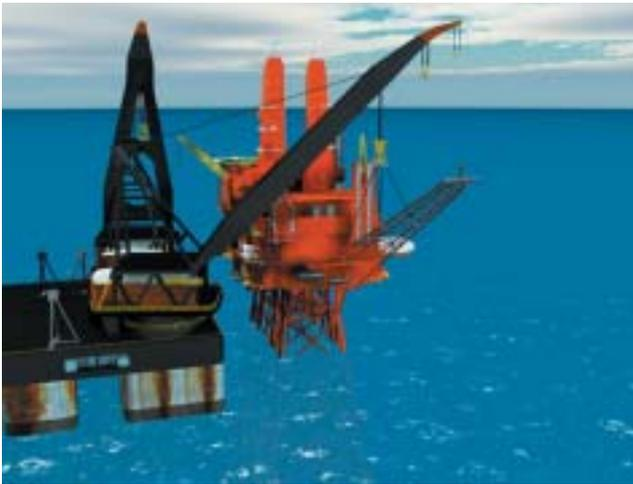
**1** Heavy lift vessel lifting the flare boom
