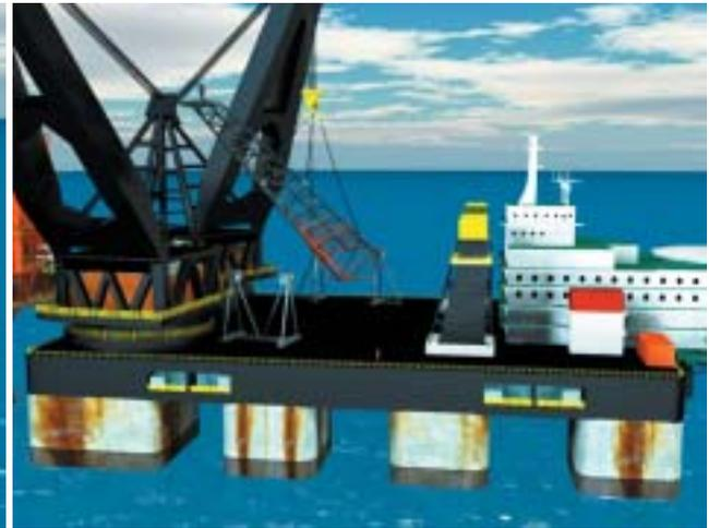
2 Flare boom being placed on the deck of the heavy lift vessel
