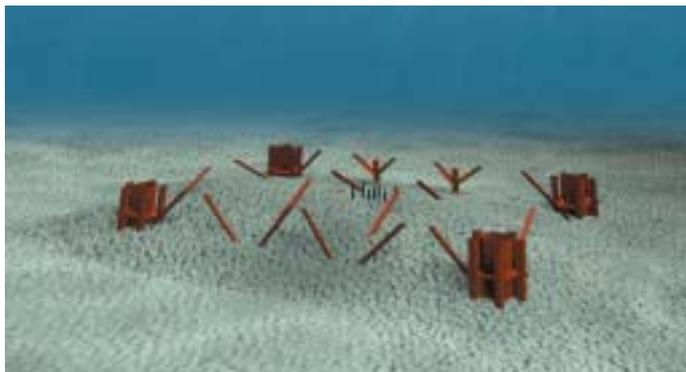
**Figure 8.3b:** Computer graphic of the North West Hutton support structure after removal of the jacket above the drill cuttings pile.
