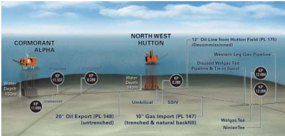
**Figure 4.6:** Layout of pipelines in the North West Hutton field.
