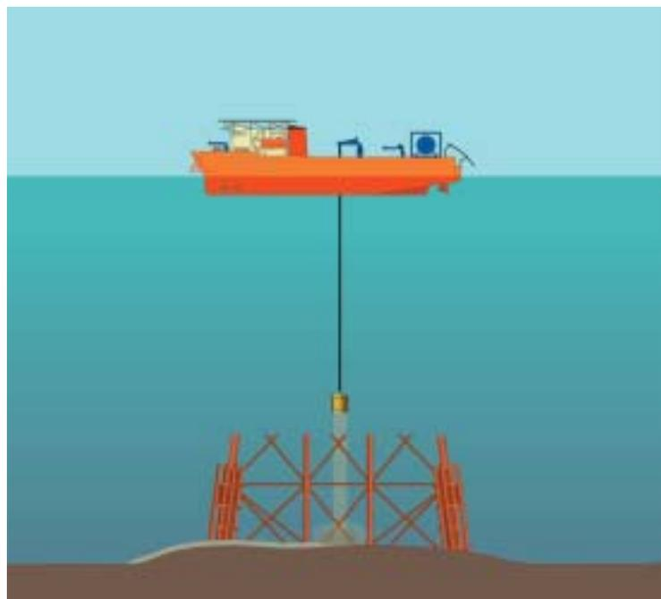
**Figure 9.6b:** Computer graphic of operations to cover the drill cuttings pile with footings in place.
