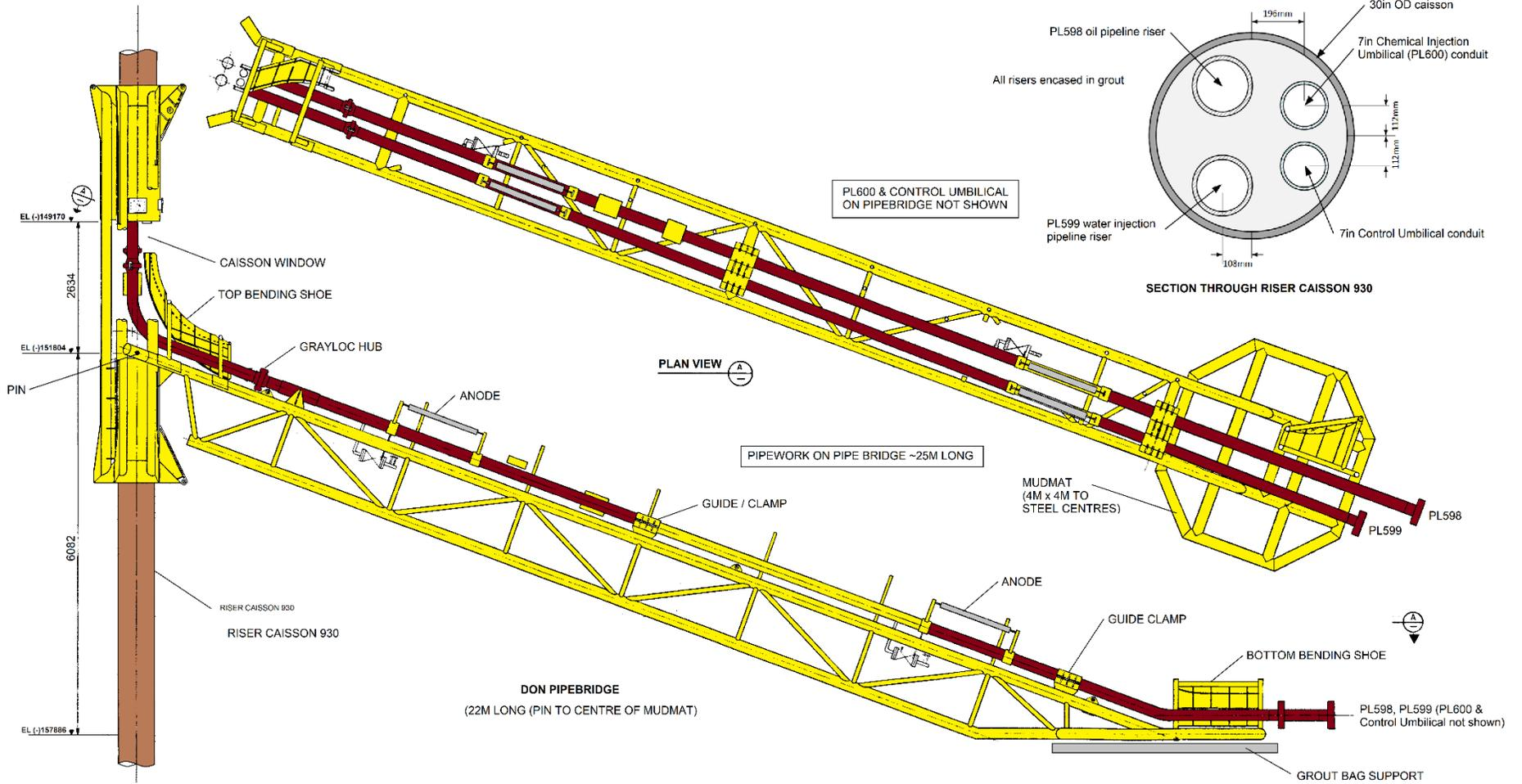
Figure 2.3.1: Don pipebridge (next to riser caisson 930 on Thistle jacket)
