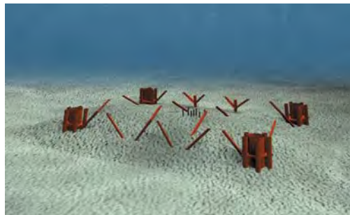
Figure 8.3b: Computer graphic of the North West Hutton support structure after removal of the jacket above the drill cuttings pile.
