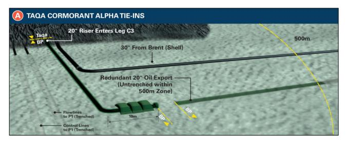
Figure 5-6 - Cormorant alpha 500m zone schematic
