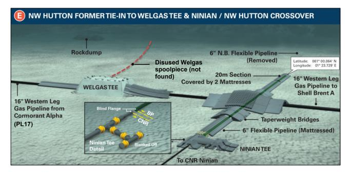
Figure 4-2 - PL 147 welgas tee area schematic
