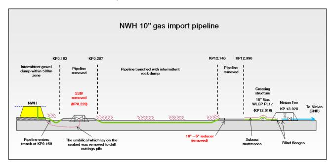
Figure 4-1 - PL147 as-left schematic
