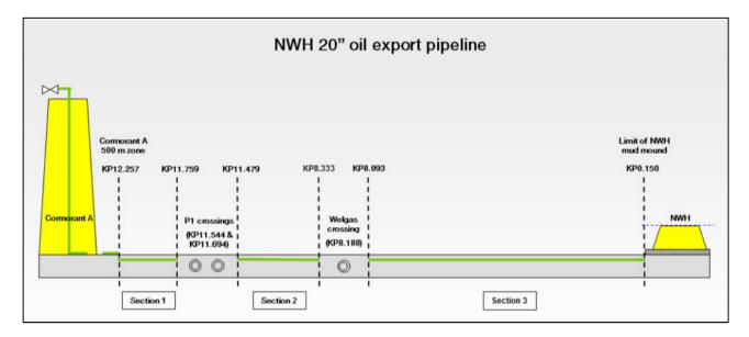
Figure 5-1 - PL 148 as-left schematic
