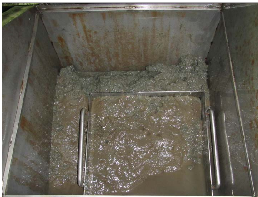
Image 2. Processing for the Gray O'Hara box core included placement of a 0.35-m × 0.35-m stainless steel insert to separate physicochemical and infaunal sediment samples.
