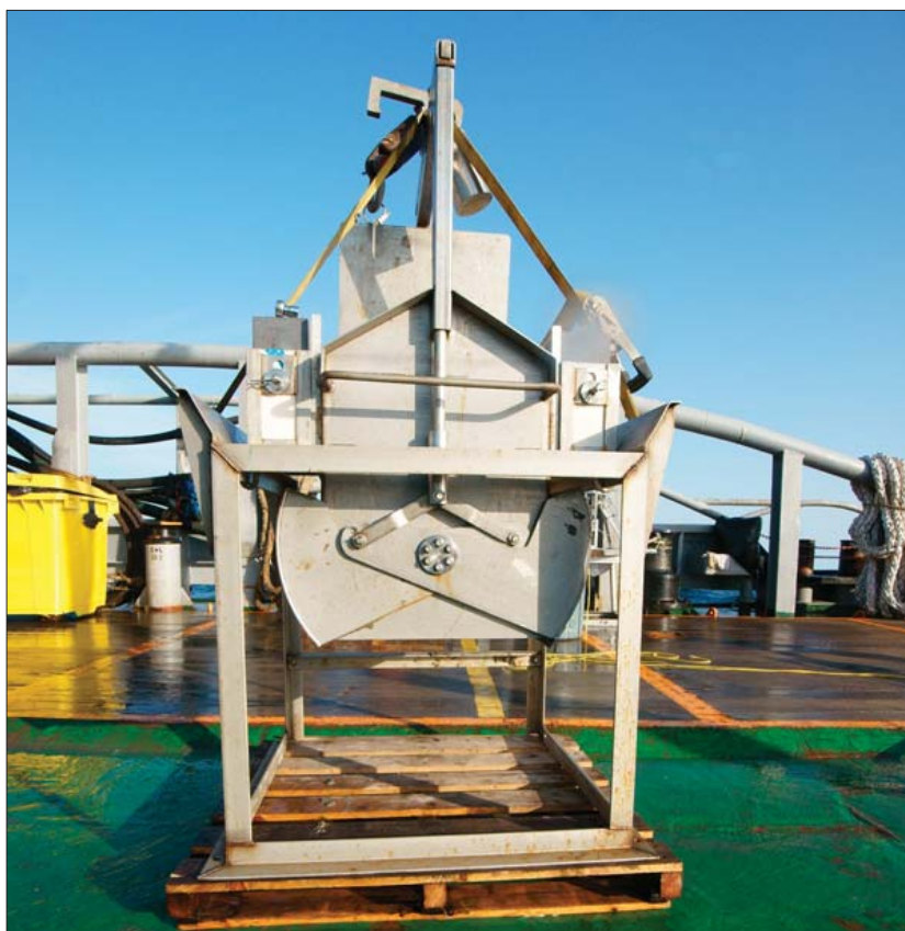
Image 1. The Gray O'Hara box core used for sediment sampling provided adequate sediment for concurrent collection of physicochemical and biological sampling parameters.
