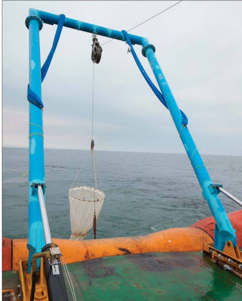
Image 5. Plankton sampling gear consisted of a 500- \mu mesh plankton net attached to a standard 1 m diameter circular, stainless steel frame. A double-trip (open-close) system was used to collect discrete-depth samples at each station.
