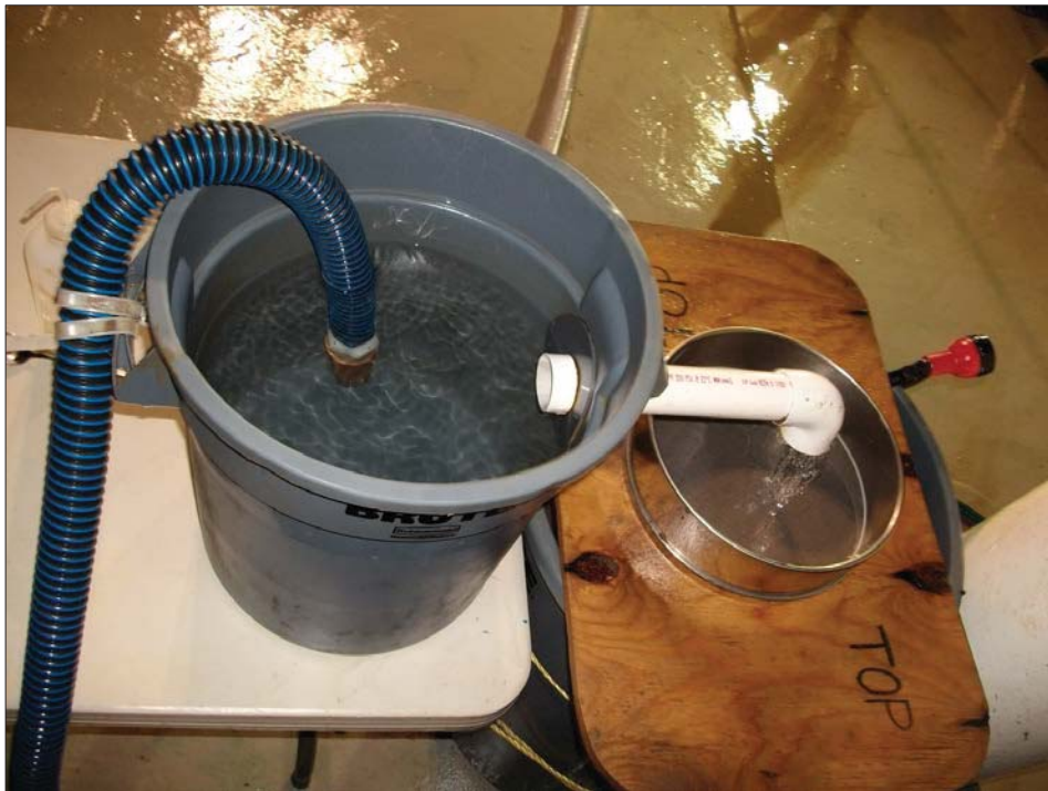
Image 3. Sediment for infaunal analysis was processed using a sieving apparatus consisting of an upper holding/flotation barrel and sieve.
