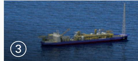
The key function of the FPSO is to remove water, condensate and reduce impurities in the gas stream before exporting processed gas to the FLNG facility and domestic gas off-take
