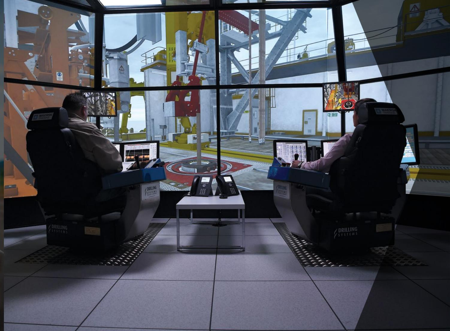
state-of-the-art simulators that can replicate nearly every critical job on an offshore drilling rig. This enables offshore teams to practice scenarios relevant to specific wells and to prepare for a wide range of contingencies.
