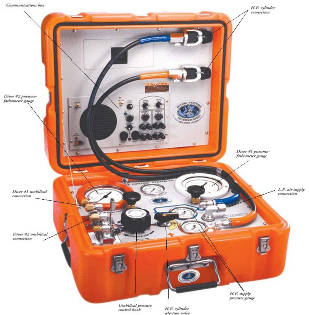
Layout of a typical diver's air manifold box. This system will accept both high-pressure and low-pressure air supplies, but only supplies low-pressure air to the diver.
