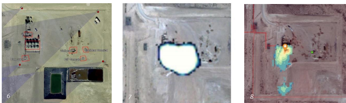
Image 6, 7, & 8: Left: Wind-cone overlay. Blue cones represent wind direction. Middle: Plume captured during aerial flyover. Right: Plume captured during satellite imaging.
